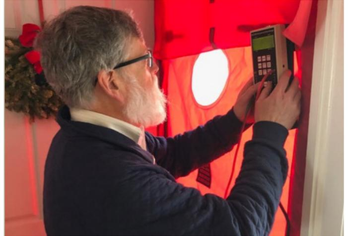
*Paul Leveille from Resilient Buildings Group, Inc. conducts a blower door test to determine air leakage.*
