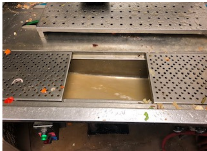
Compostable waste enters the pulping tank via a trough where it mixes with water and is ground into a slurry.
